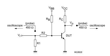
$$\begin{split} &V_i = 9.5 \; V; \; T = 500 \; \mu s; \; t_p = 10 \; \mu s; \; t_r = t_f \leq 3 \; n s. \\ &R1 = 68 \; \Omega; \; R2 = 325 \; \Omega; \; R_B = 325 \; \Omega; \; R_C = 160 \; \Omega. \\ &V_{BB} = -3.5 \; V; \; V_{CC} = 29.5 \; V. \\ &Oscilloscope: input impedance \; Z_i = 50 \; \Omega. \end{split}$$
